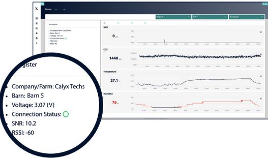
**1** Check the Y-series battery capacity from the Calyx Connect webpage. Make sure the battery voltage is larger than 3.00 V.
